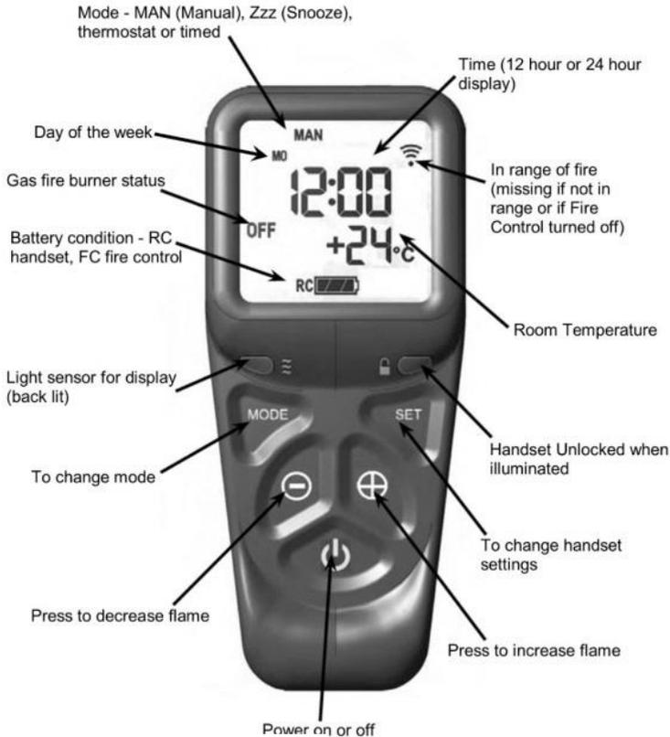
Fig.4 Remote control handset
