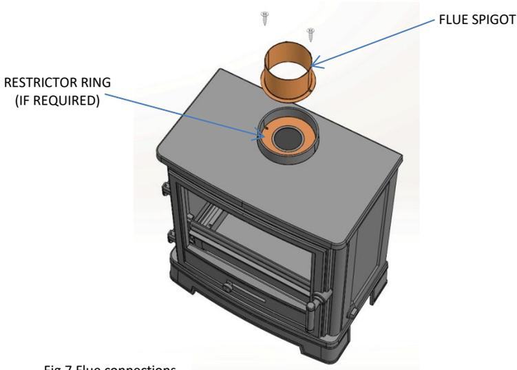
Fig.7 Flue connections
