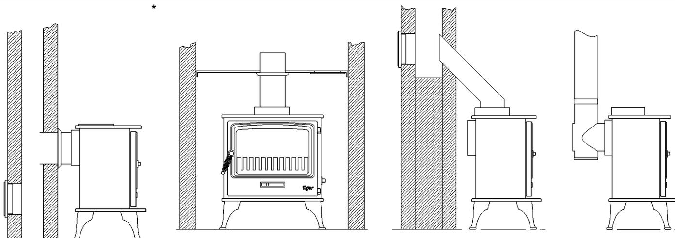
Rear flue connection into chimney with sealing collar. Cleaning door on opposite side.
