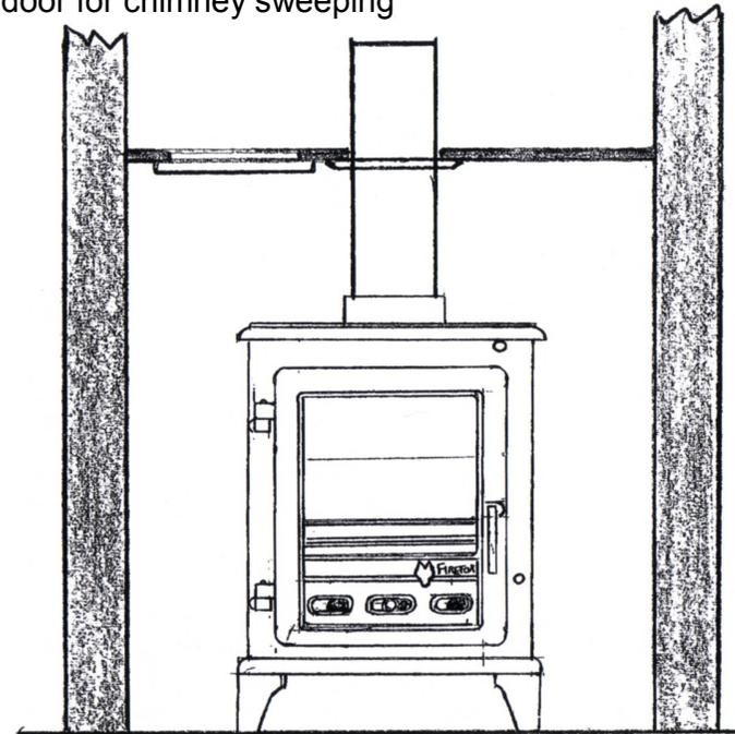
**Typical Rear Flue Installation** with clean out door
